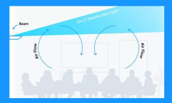
Upper room ultraviolet germicidal irradiation (UVGI) is an air disinfection method generally recommended by ASHRAE and the CDC. R-Zero's upper room UVGI solution, Beam, has been independently validated for its ability to inactivate microorganisms, including:
