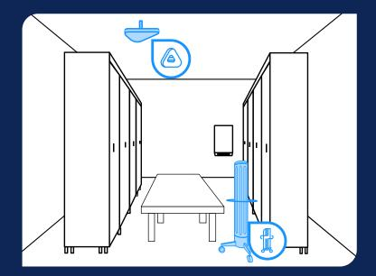
Far-UV disinfection can provide continuous disinfection of handles, locker surfaces, and the floor, prevent mold and mildew from taking hold within lit areas, and inactivate mold spores in the air. A regular mobile tower UV disinfection cycle can supplement this with high-power light into open lockers and in shower areas. For custodial staff, this can reduce the frequency and time required for disinfection.
